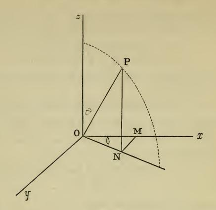
plane of zx. These are called the polar co-ordinates of P and are usually denoted by the letters r,  $\theta$ ,  $\phi$ . They are connected with the rectangular co-ordinates of P referred to the axes Ox, Oy, Oz by very simple relations which can be obtained thus. Draw PN parallel to Oz to meet the plane of xy in N, and NM parallel to Oy to meet Ox in M. Join ON.
